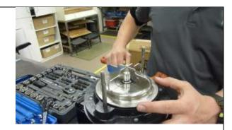
5. Lifting the pump case off the shaft.
