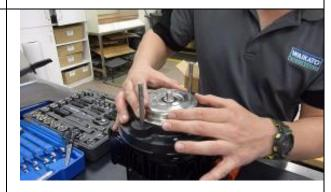
6. Next, take out the seal and spring then clean the cavity before reassembly with the new seal. The seal inside the pump case is tapped out with a soft hammer handle, the space cleaned and lubricated to fit the new seal.
