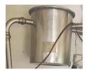
**Receiving Can:** Milk flows into the receiving can from the milk line under vacuum and from here is sucked out by the milk pump into the milk vat or can.
