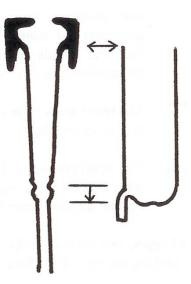
**Teat Cups:** Hold the liner in place allowing the vacuum and pulsation to squeeze the liner in and out to extract the milk.
