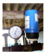
**Vacuum Can/Reserve Can:** Allows a reserve of vacuum to allow for loses due to air getting in due to cup changing, cups being kicked off or rubbers coming off. Without this reserve every time a small amount of air gets in the vacuum would drop too low and set of cups would fall off.
