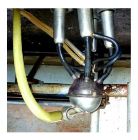
**The air admission hole:** This tiny hole in the claw, 0.8 to 1.0 mm in diameter, allows air into the claw to drive the milk up to the milk line.
