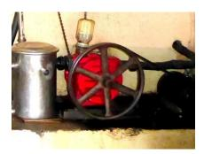
**Oiler:** Distributes oil into the vaccum pump to lubricate the veins inside it that move in and out to create the vaccum
