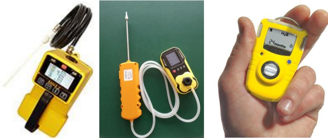
Figure 3.2 Typical portable biogas/hydrogen sulphide safety detectors
